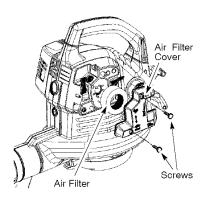
A dirty air filter decreases engine performance and increases fuel consumption and harmful emissions. Always clean after every 5 hours of operation. Cleaning the air filter:
